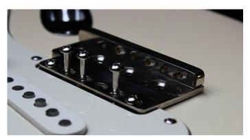
Scrape a bit of candle wax on the four inner bearing screws before screwing them down as normal until they just touch the surface of the plate ( when flat). Just ensure they are not gripping the plate.
