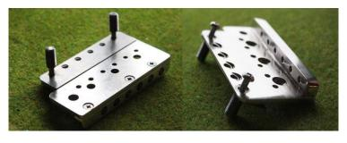
Simply place the bridge unit into the trem rout in the body and locate the two outer screws (which screw directly into the shanks in the body). Place a couple of business cards, approx the same .5mm thickness as the shim at the front, under the back edge of the plate to protect the body. Bring the screws down a few turns on each side at a time, until the plate is sitting
