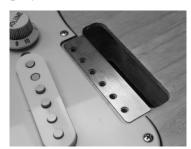
Using the shim as a template, carefully cut around the edge with a sharp stanley knife.
