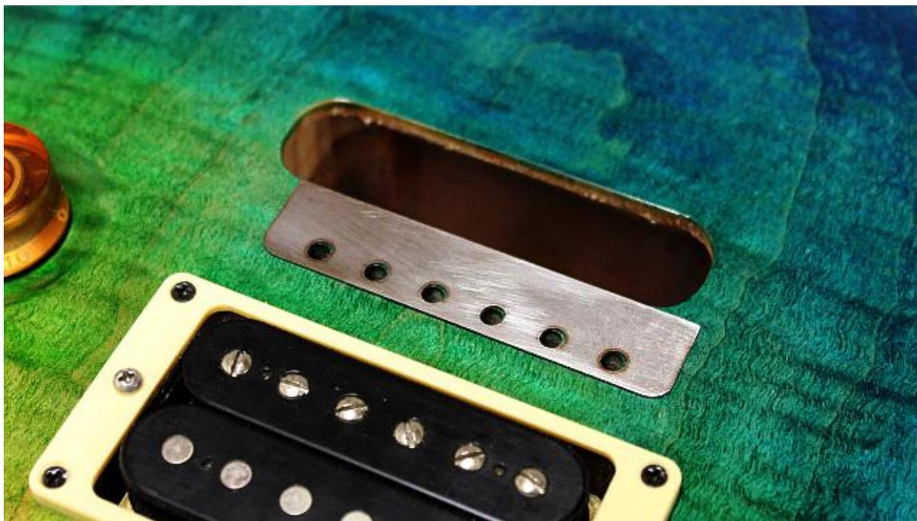
Then place the Wudtone Tremolo unit in position on top of the shim. With or without saddles fitted it doesn't matter.
