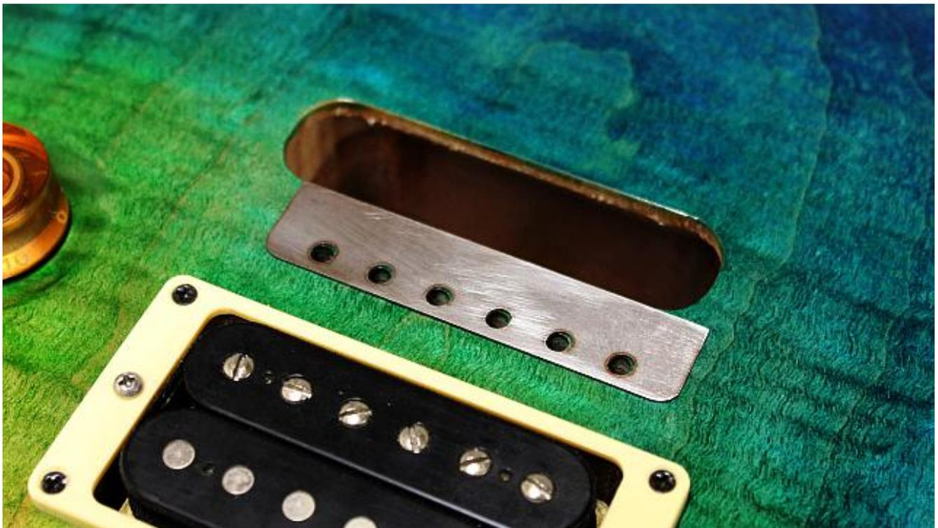
Then place the Wudtone PRD DD tremolo unit in position on top of the shim. With or without saddles fitted it doesn't matter.
