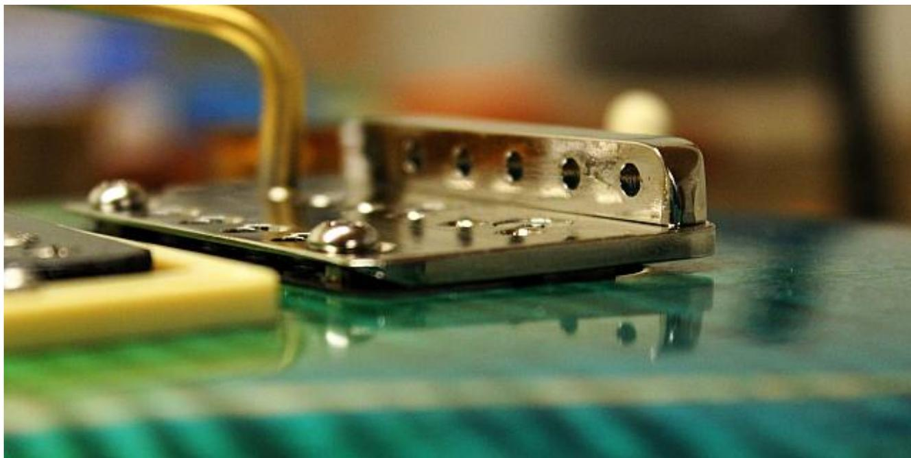
Experiment , slightly over tightening each screw and then backing off. Too tight and the plate will be lifted too much at the back edge. Too slack and the plate will be lower at the back edge and so at more than 90 degrees to the bearing screws.
