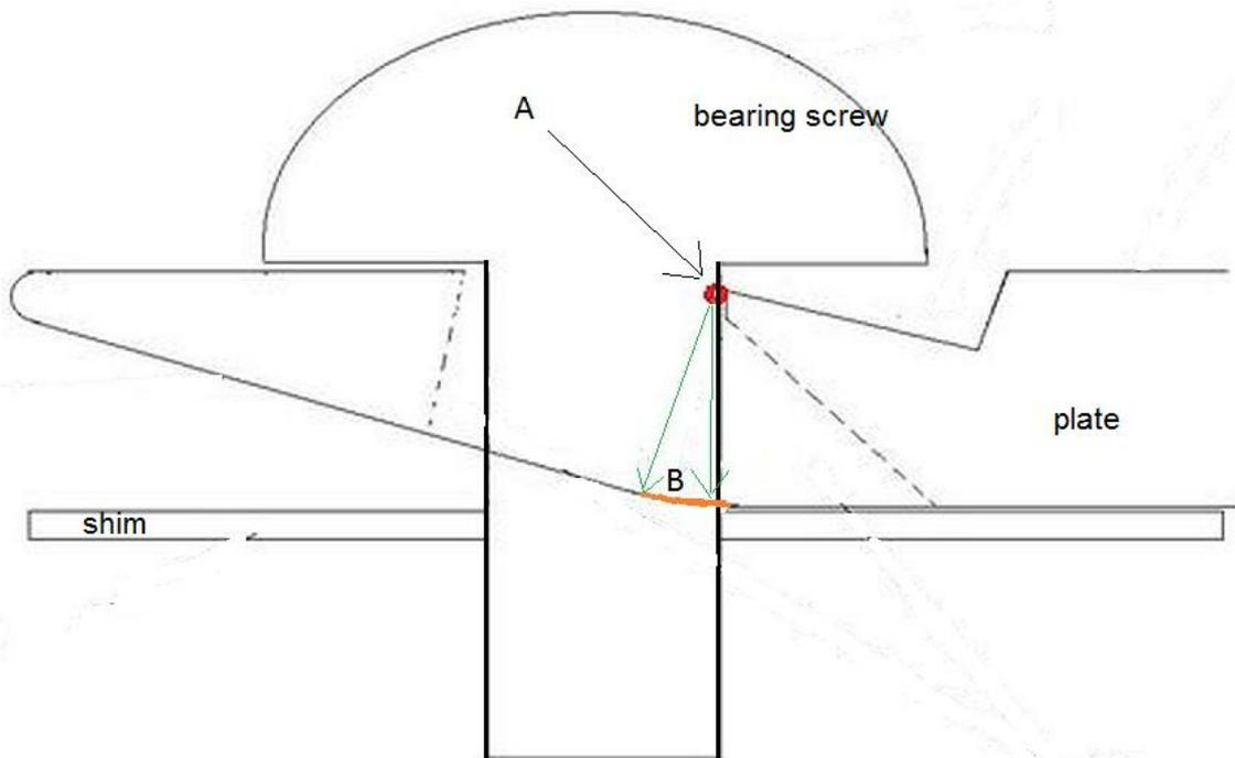
Before any springs or strings are fitted , it is important to set correctly the height of each bearing screw.
